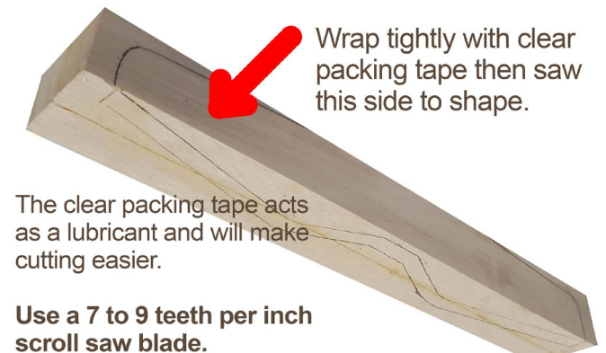
STEP 18: Tape both ends and middle of the 3 sawn pieces shown in STEP 16 and 17. Next, scroll out the top shape of the wing for both wing parts B1 and B2 as shown in STEP 19 page 7.
